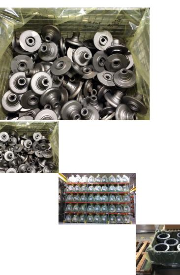
ZERUST®/EXCOR® ICT®510C-AN Film utilizes Vapor Corrosion Inhibitor Technology (VCI) to protect metals in challenging situations. It is effective on metals that may be difficult to protect, such as highly porous and powdered metal parts.
